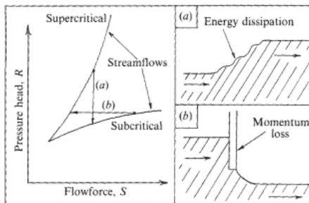
FIGURE 1. Flow transitions in the  $(R, S)$ -diagram: (a) the bore, (b) the sluice (or hydroplane).
